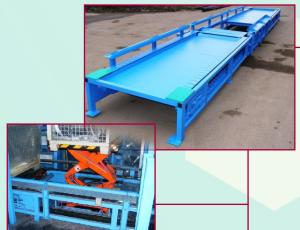
The conveyors DPH without belts are used for transport of loose materials. The conveyor may be designed in L or Z shape. The chain drags rakes along the metal sheet trough of the conveyor structure and carries the transported material.
